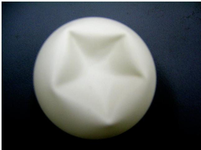
Fig. 8. Ping pong balls are good macroscopic examples for shells as they display the main features of shell deformation (linear elastic response at deformations in the order of the wall thickness followed by buckling instabilities at larger deformations). Image courtesy S. Komura, (Tokyo Metropolitan Univ, Fac Sci, Dept Chem, Tokyo 1920397, Japan).
